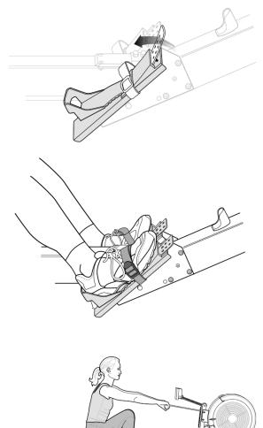
To set the Flexfoot, pull the toe piece toward you to release the flexfoot from the two pegs. Slide the toe piece up or down to achieve the proper setting, then press the toe piece back down onto the pegs.
